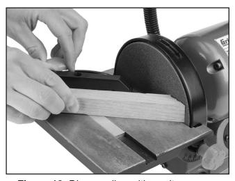
Figure 12. Disc sanding with a miter gauge.
